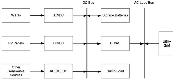
Fig. 1. Configuration of a typical hybrid generation system.
