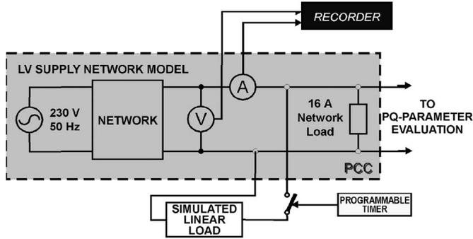
Fig. 13. Representation of the simulated setup used for the analysis of the influence that a change of the magnitude of the network impedance may have on the measurement of flicker.
