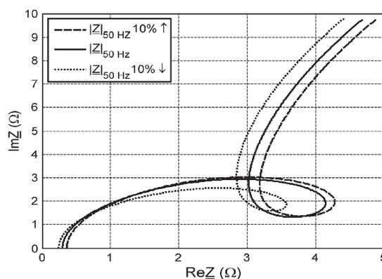
Fig. 7. Change of the complex network impedance plot when  $|Z|$  at 50 Hz changes with  $\pm 10\%$ .
