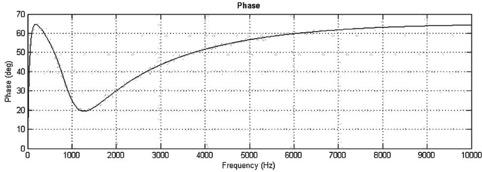
Fig. 3. Variation of the phase of the network impedance with frequency.
