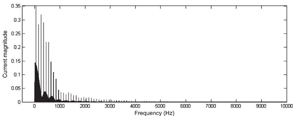
Fig. 6. Frequency-domain representation of the distorted current induced by the SMPS.
