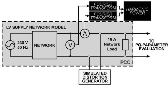
Fig. 12. Representation of the simulated setup used for the analysis of harmonic power distortions.
