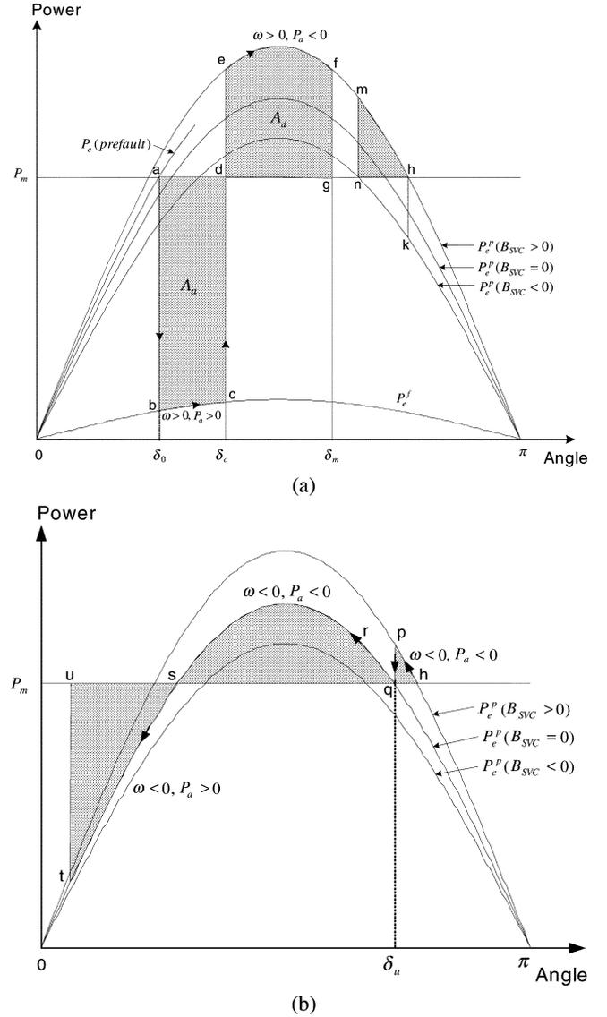
Fig. 3.  $P-\delta$  curves for various operating conditions of SVC: (a) areas when the angle increases and (b) areas when the angle decreases.
