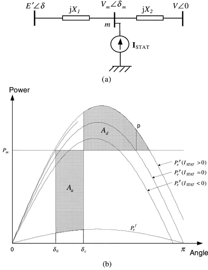
Fig. 5. System with a STATCOM: (a) equivalent circuit and (b)  $P-\delta$  curve.
