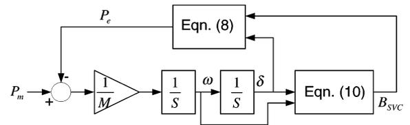
Fig. 4. Simulation block diagram of the system with a SVC.
