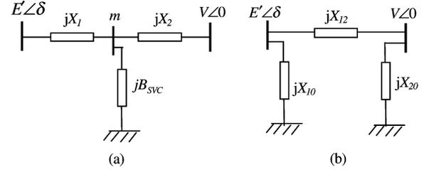
Fig. 2. A SMIB system with a SVC.
