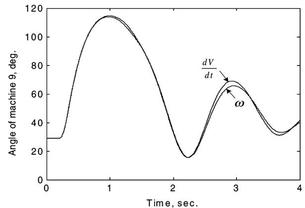
Fig. 14. Swing curve of the most severely disturbed machine (machine 9) obtained by using  $\omega$  and  $-dV/dt$  as control signals.
