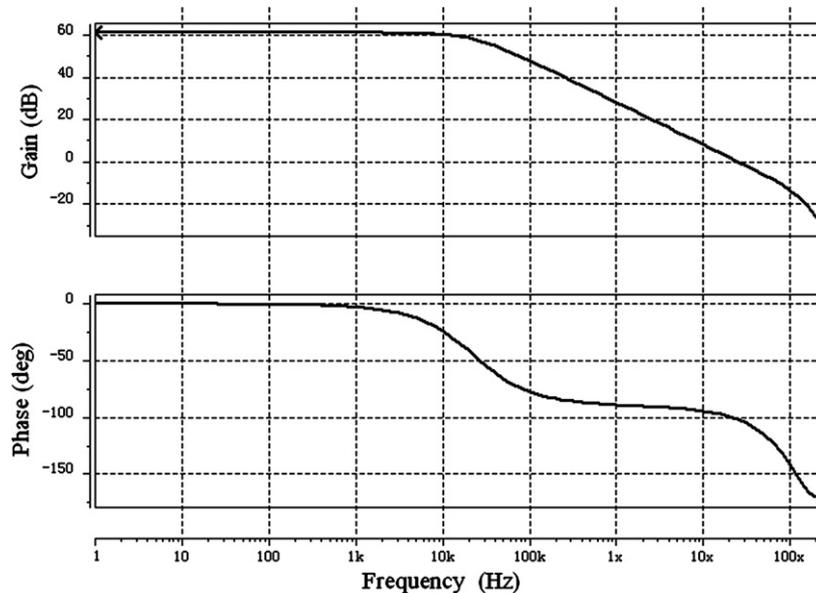
Fig. 8. AC response of the single stage amplifier.
