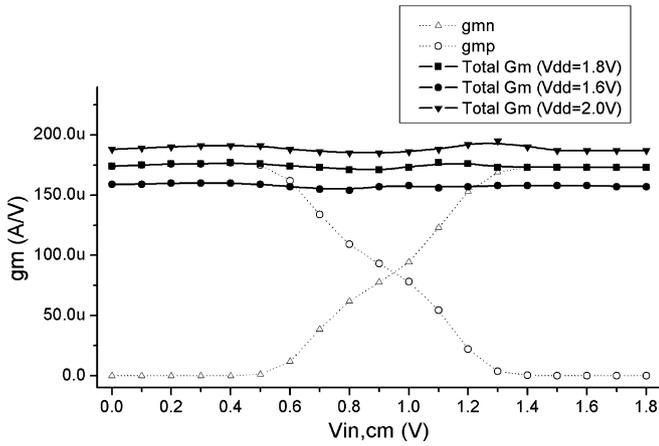
Fig. 6. Simulated  $g_m$  vs.  $V_{icm}$  of the input stage under different supply voltages.
