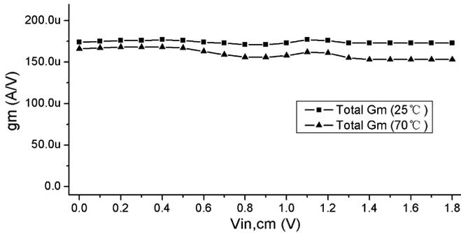
Fig. 7. Simulated  $g_m$  vs.  $V_{icm}$  of the input stage under different temperatures.
