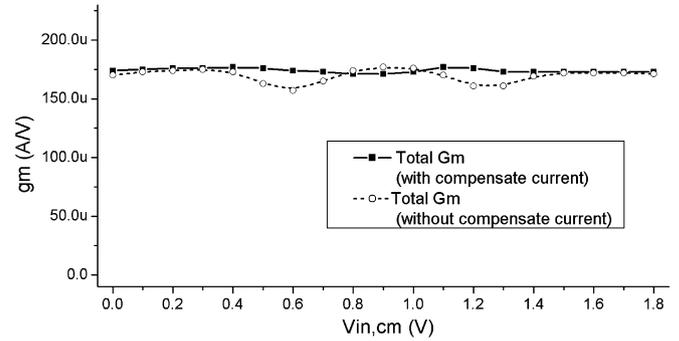
Fig. 5. Compare the  $g_m$  variation vs.  $V_{icm}$  of the circuit between with and without compensate current.
