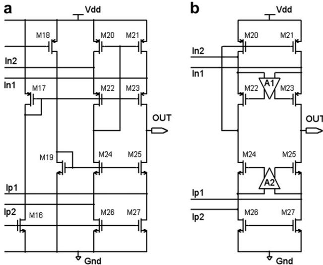
Fig. 3. (a) Folded cascodes summing circuit and (b) gain boosting technology implements in (a) for higher gain.
