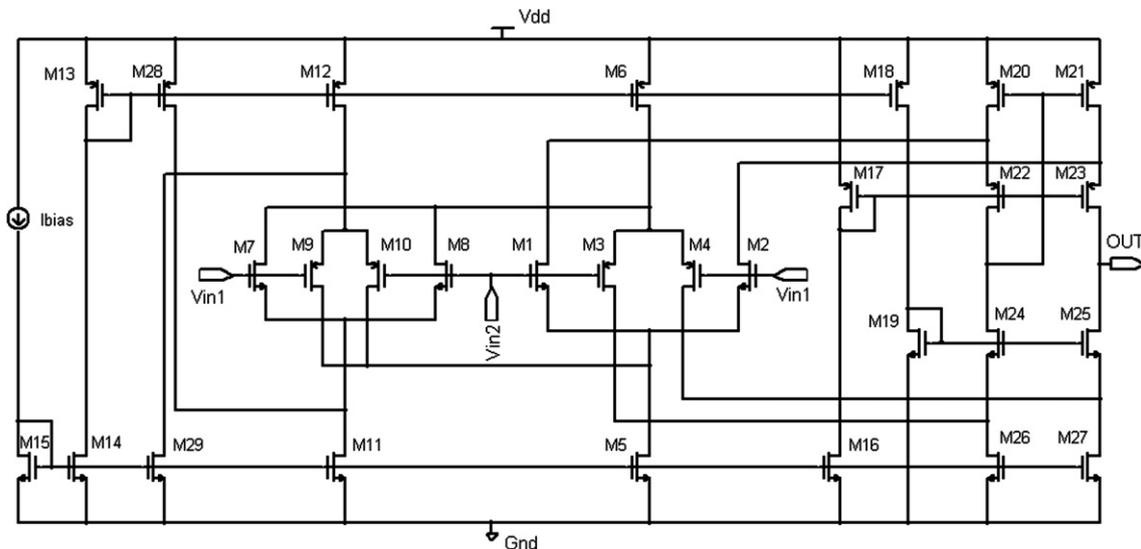
Fig. 4. Overall design of constant- $g_m$  rail-to-rail Op Amp input stage.
