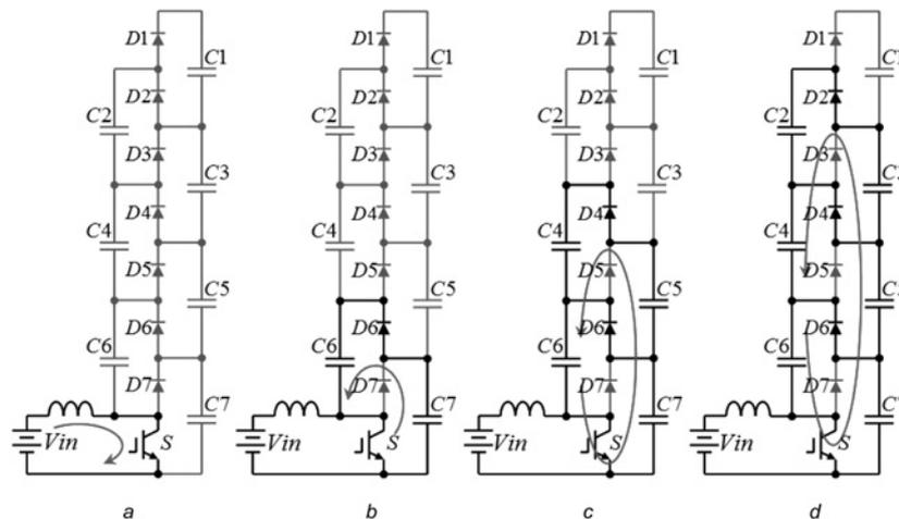
Figure 3 Switch-on state
