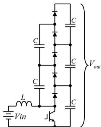
Figure 10 Prototype schematic:  $L = 1.33 \text{ mH}$ ,  $C = 100 \mu\text{F}$
