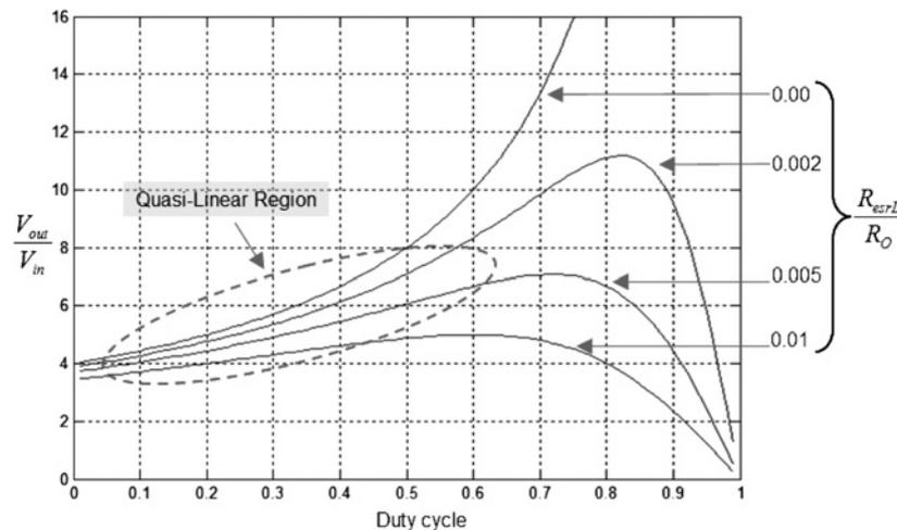
**Figure 5** Voltage gain against duty cycle for different values of  $ESR/R_O$  in the novel MBC ( $N = 4$ )
