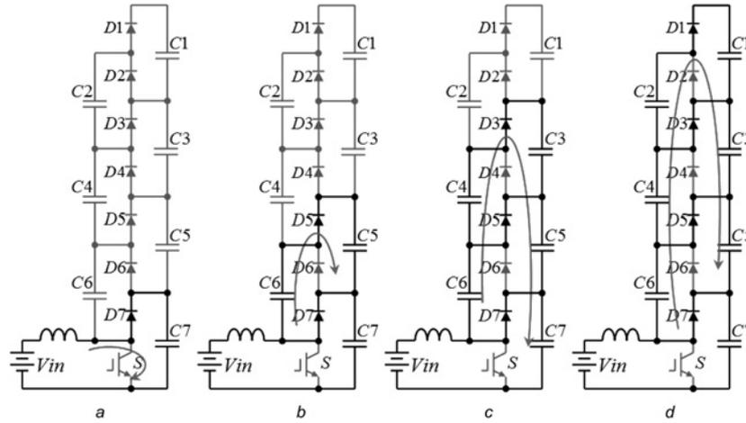
Figure 4 Switch-off state
