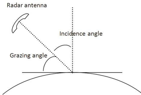
**Fig. 3.** Geometry of a marine radar
