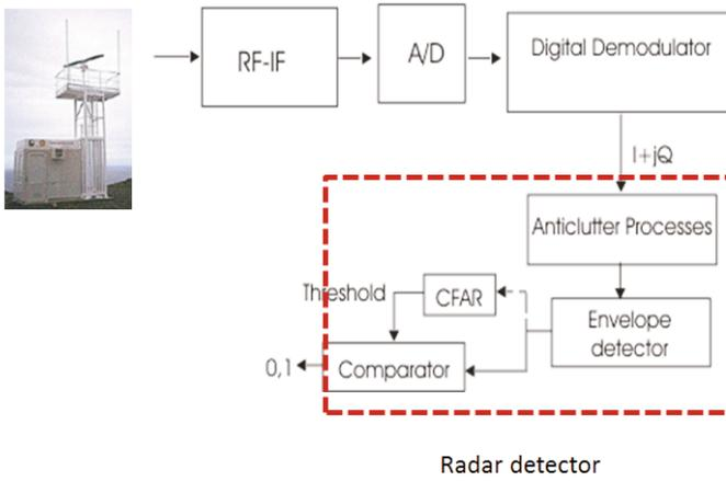
**Fig. 1.** General architecture of a coherent radar
