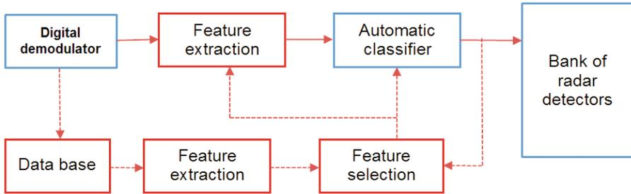
**Fig. 5.** Proposed detection scheme based on a bank of detectors and a clutter classifier capable of selecting the more suitable detector among those available
