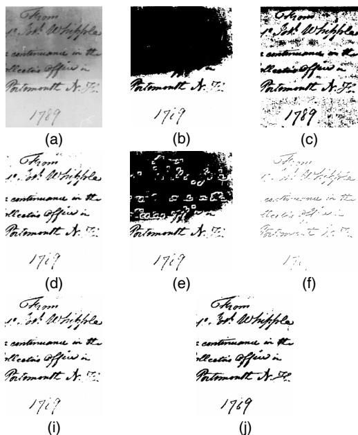
Figure 5. Binarization results: (a) Original image; (b) Otsu's approach [1]; (c) Niblack's approach [3]; (d) Sauvola's approach [4]; (e) Bernsen's approach [2]; (f) Adaptive Logical approach [5]; (i) Adaptive degraded document approach [6] and (j) the proposed approach.
