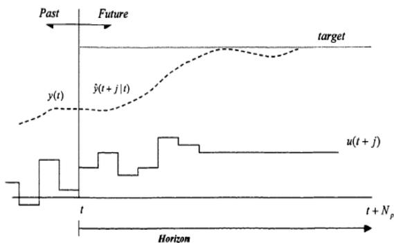
Figure 2: Moving horizon approach of Model Predictive Control
