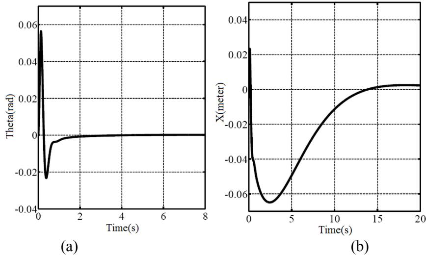
Figure 7. The time responses of Inverted Pendulum system while the pendulum’s angle is controlled beneath the cart’s position. a. Time response of pendulum’s angle. b. Time response of cart’s position.
