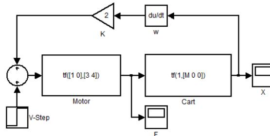
Figure 2. MATLAB simulink diagram for determining the motor's constant (k), in which we have the cart's approximate transfer function and the motor's proposed one.
