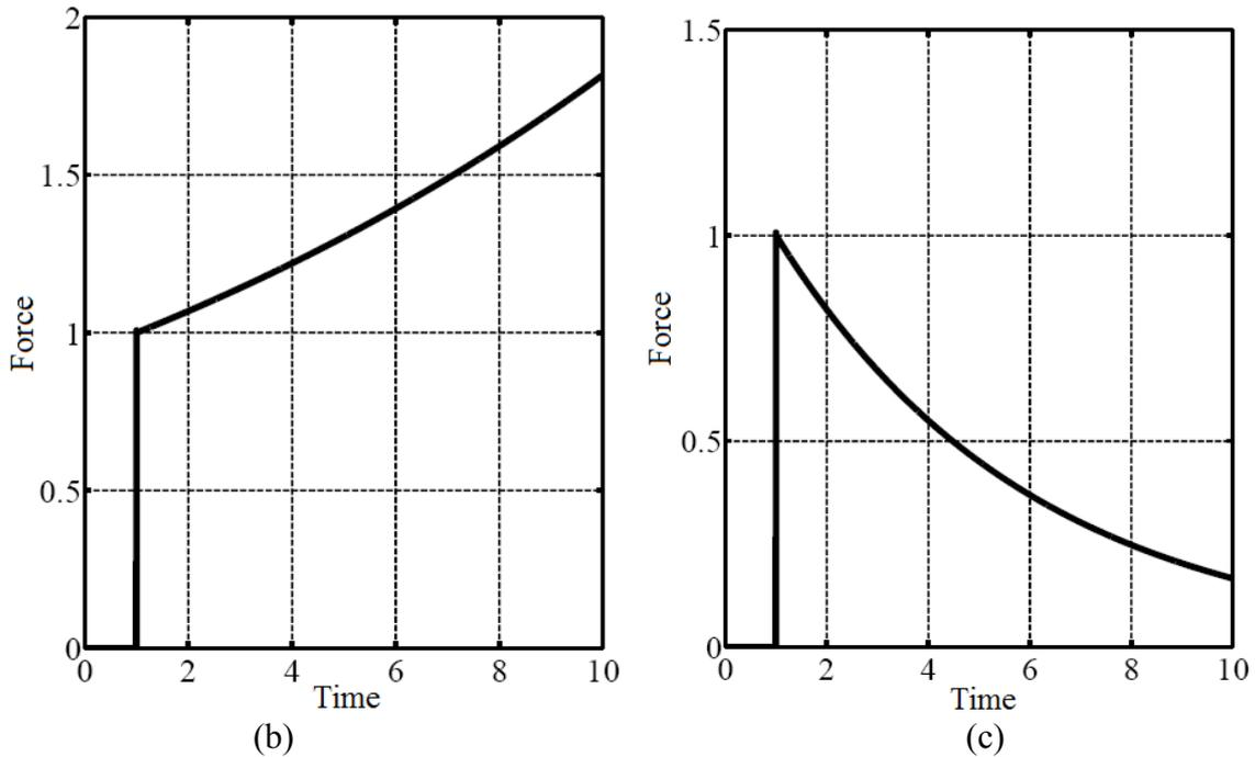
Figure 3. Motor's time response to a constant applied voltage in different values of k. (a.  $k=2$ , b.  $k>2$ , c.  $k<2$ )
