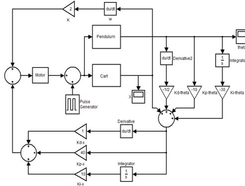
Figure 6. MATLAB simulink diagram in order to control the pendulum's angle beneath cart's position.
