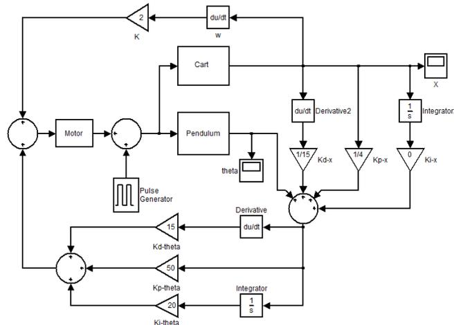
Figure 4. MATLAB simulink diagram in order to control the cart's position beneath the pendulum's angle.
