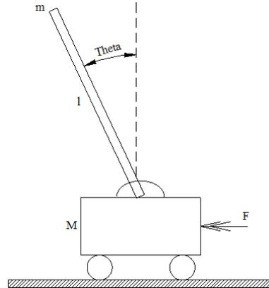
Figure 1. Inverted Pendulum's free diagram
