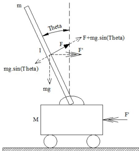
Figure 8. Inverted Pendulum’s free body diagram and the applied forces in order to compensate for the nonlinearity trait.
