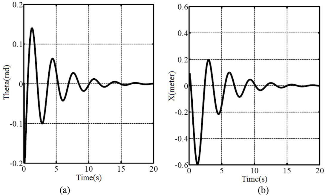
Figure 5. The time responses of Inverted Pendulum system while the cart's position is controlled beneath the pendulum's angle. a. Time response of pendulum's angle and b. Time response of cart's position.
